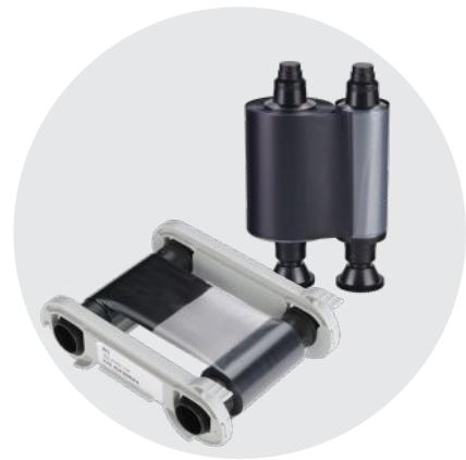
The Evolis High Trust® KO ribbon has been specifically engineered to bring durability to monochrome personalization. The KO ribbon has 2 panels; a black panel (K) to print black text or barcode, and a clear overlay panel (O) to apply a thin protective film.
