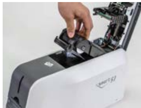
Figure 19 Installing the ribbon cartridge
