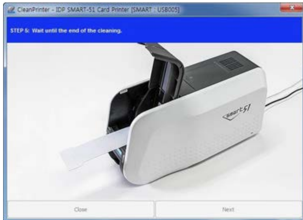
Figure 110 Printer cleaning Step 5
