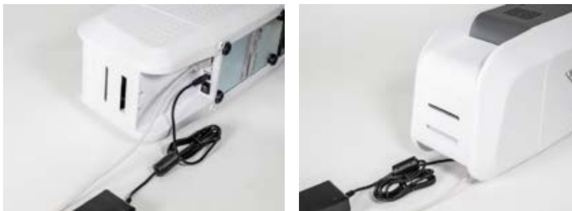
Figure 10 SMART-51D Connection of power and USB cable
