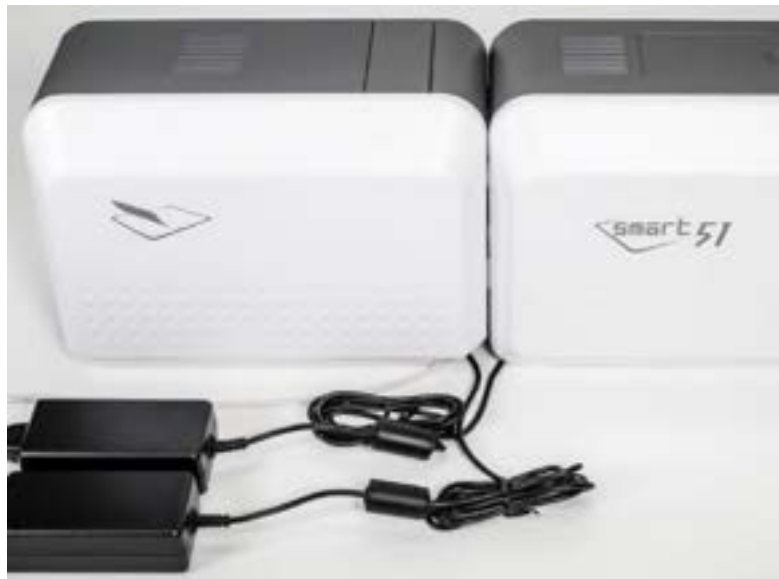
Figure 12 SMART-51L Connection of powers and USB cable - 2
