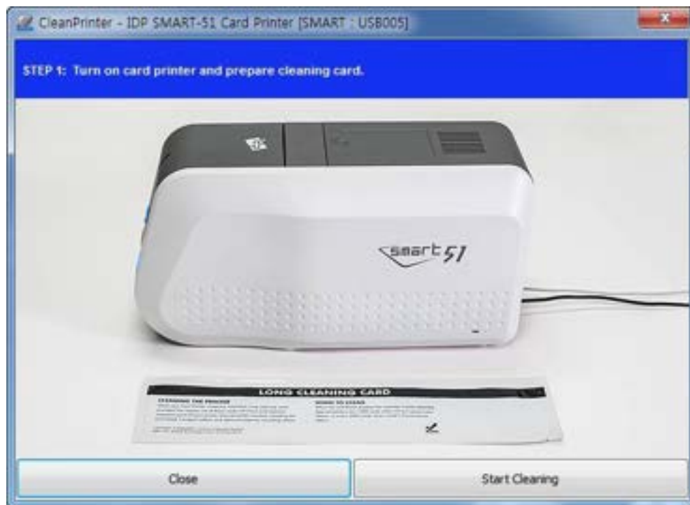
Figure 106 Printer cleaning Step 1
