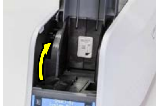
Figure 24 Adjusting the card thickness lever
