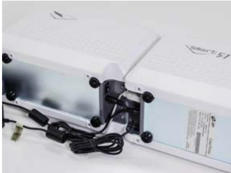
Figure 11 SMART-51L Connection of powers and USB cable - 1
