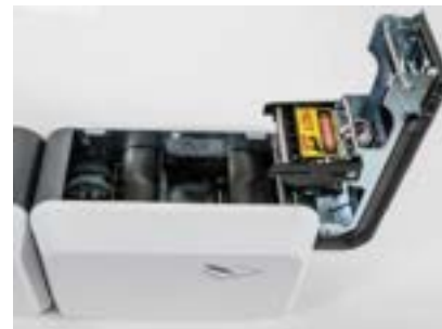
Figure 23 Installing the film cartridge
