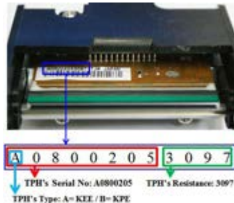
Figure 112 Thermal Print Head
