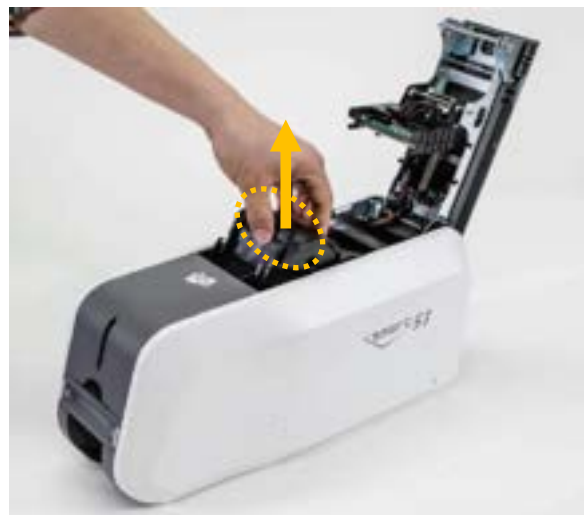
Figure 14 Take out the ribbon cartridge
