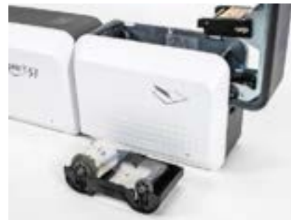
Figure 22 Loading the laminating film
