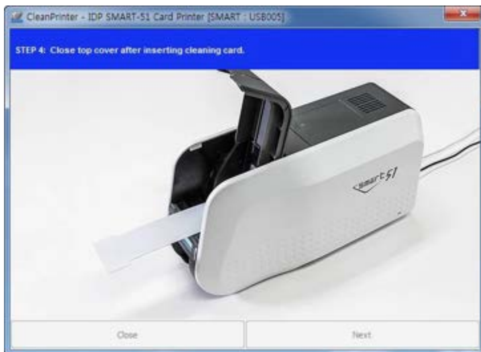
Figure 109 Printer cleaning Step 4
