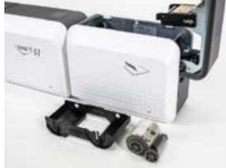
Figure 21 Take out the film cartridge
